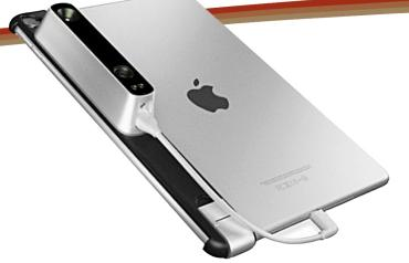
The Allied OSI iPad Scanner allows you to scan for custom orthotics instead of using plaster or foam molds.
